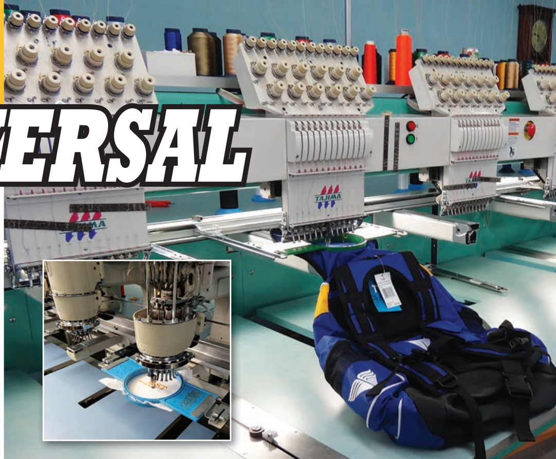
The embroidery room has a total of 21 machines to embroider logos on caps, bags, T-shirts, etc. The normal amount of stitches for each machine to run is 600 stitches per minute.
