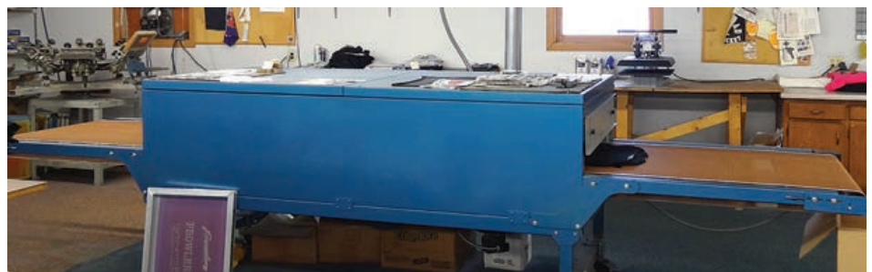
Silk screening of T-shirts and numerous other items are done on a series of plates that rotate from a central pivot. The shirts are then put into an oven to allow the paint to dry and cure at the proper temperature.
