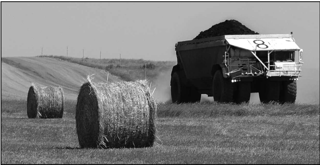
One of BNI Coal's eight Kress trucks drives toward the Young Station with a 180 ton load of coal.
