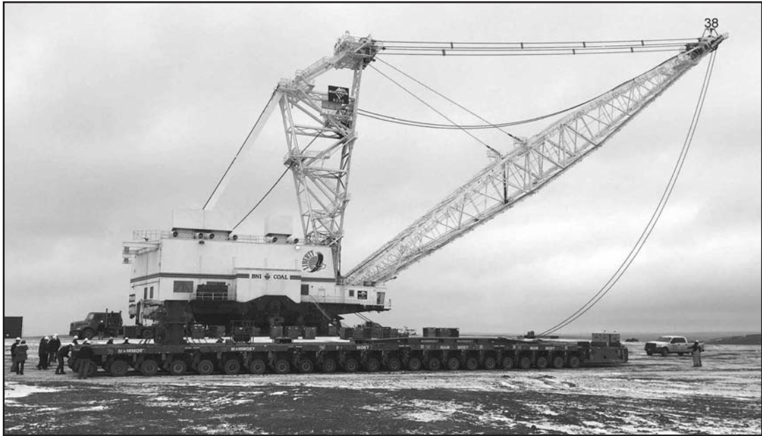
The Liberty dragline was transported eight miles to its new home in February using self-propelled modular transporters.
