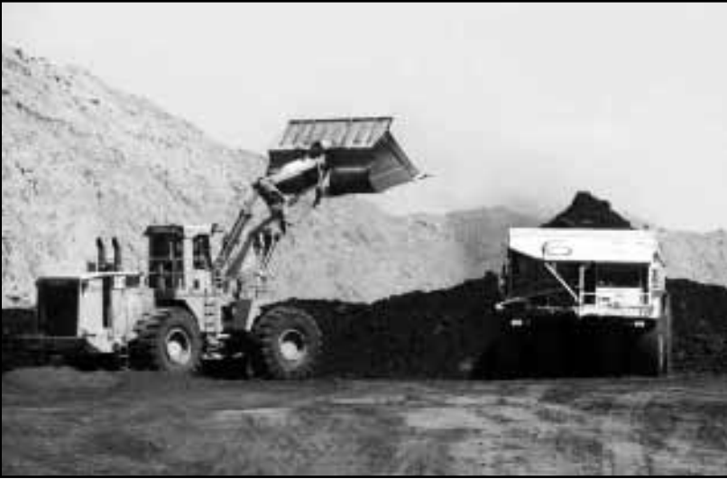
A 992G Caterpillar front-end loader equipped with a 30-cubic yard bucket loaded lignite coal into a CH180 Kress unibody diesel coal truck. BNI Coal operates six of the Kress trucks, each capable of hauling 180 tons of lignite. The two coal-fired generating plants of the Milton R. Young Station require 4.5 million tons of coal per year. BNI delivers coal at a cost of $15 a ton for an annual cost of $67.5 million.
