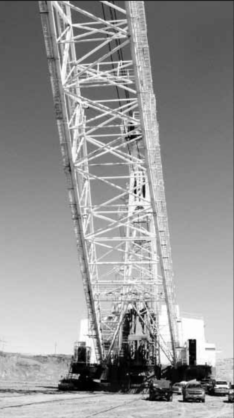
Pictured is "Liberty" an 8200 Bucyrus electric dragline that is used by BNI Coal to remove overburden to expose the lignite coal seams. Liberty was commissioned in 2004. It weighs 9,257,000 pounds, has a 355-foot boom and a 77 cubic yard bucket. It is the newest and largest operating dragline in North America.
