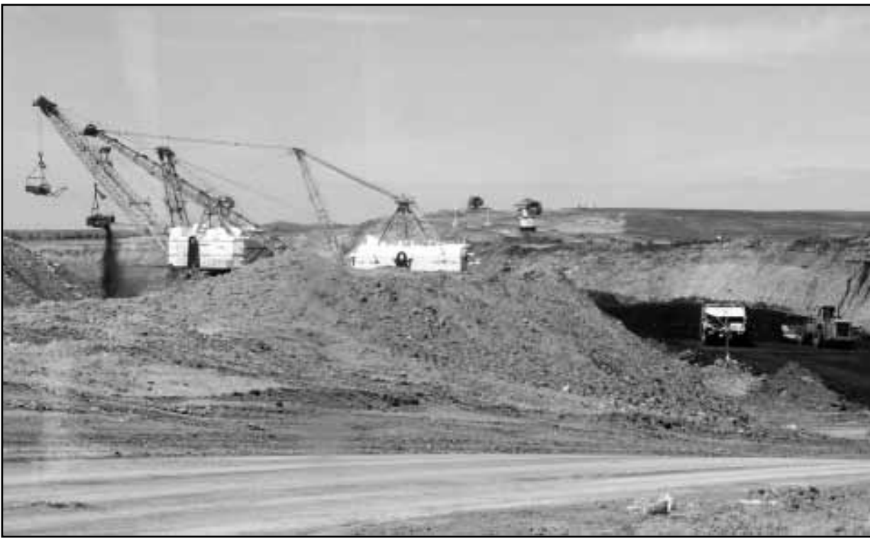
Two smaller Page electric draglines are also used to strip overburden from the lignite coal seams. In the mining operation, 30 million cubic yards of earth are moved each year. The replacement cost of all the equipment used by BNI Coal would be approximately $155 million.
