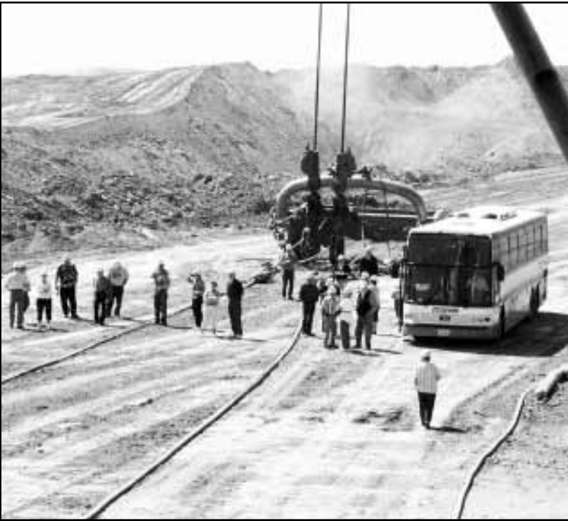
This picture taken from inside the operator's cab of "Liberty", shows how the 77 cubic yard bucket compares in size to a 50-plus passenger charter bus.
