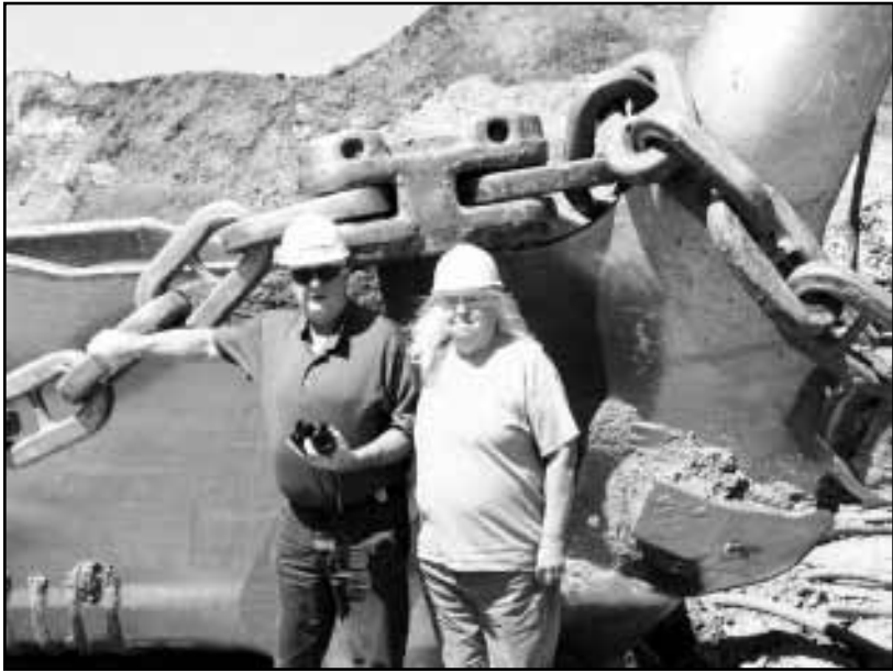
Steve and Ruth Sundbom of Clearbrook stood in front of the 77 cubic yard bucket used on the large "Liberty" dragline. The bucket has a 385,000-pound "Rated Suspended Load". Replacement buckets cost $1 million and are built in Australia. BNI Coal has two spare buckets in stock at all times.
