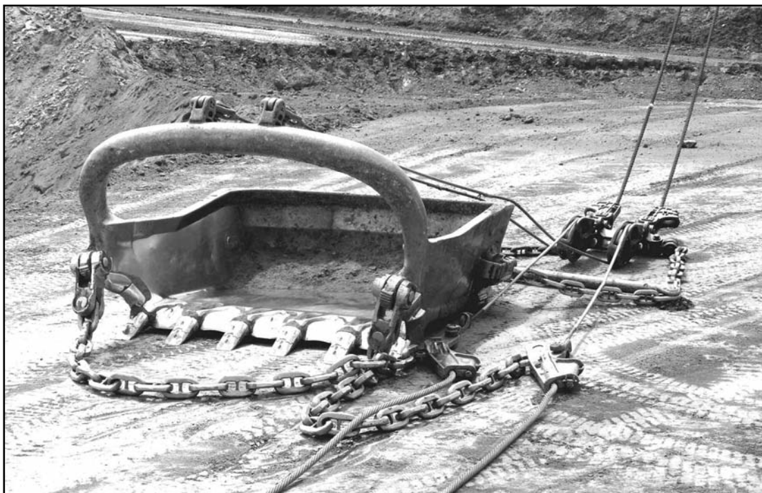
The bucket of the Bucyrus dragline has a 77 cubic yard rating. When empty it has a weight of 150,320 pounds. With the tour participants on the dragline, while it was operating, one of the bucket loads registered 88 cubic yards.
