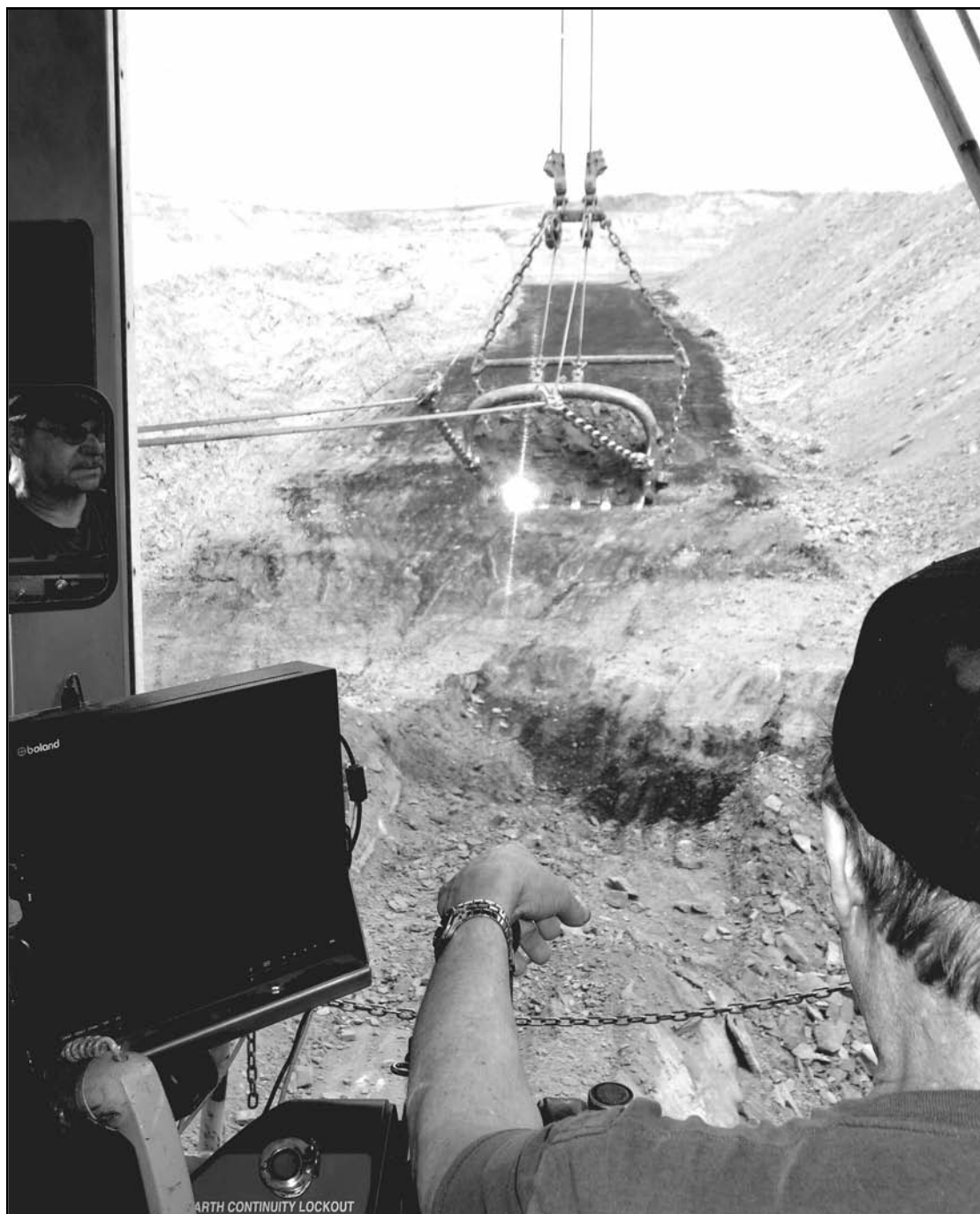
This photo overlooks the shoulder of the Bucyrus dragline operator as he operated the bucket of the dragline. In a typical eight hour shift, 300 to 330 buckets of overburden will be moved. The computer screen on the left records the weight and time duration of each bucket load.
