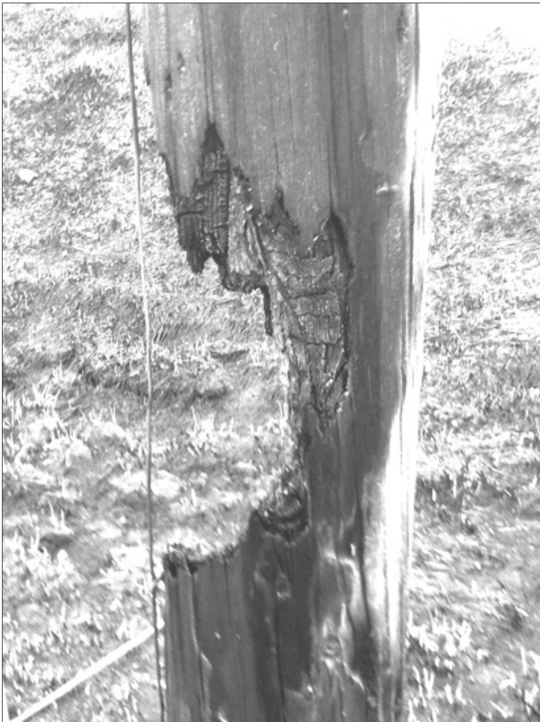
Damaged electrical pole after controlled burn went out of control.
