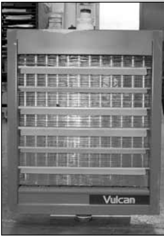
Lots 4 and 5: Vulcan steam or hot water unit heater, new in 2004. Steam output is 60,000 BTU; hot water output is 43,000 BTU. 1/20 HP 115V fan motor.
