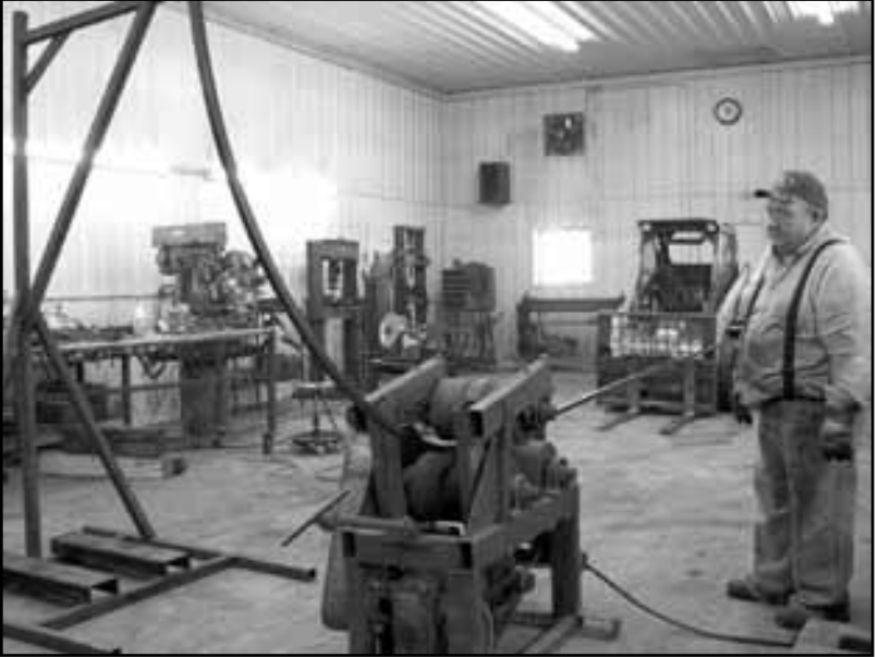
Rodney Burns bends a 14-gauge steel tube that is used to make hay rings and cattle feeders.
