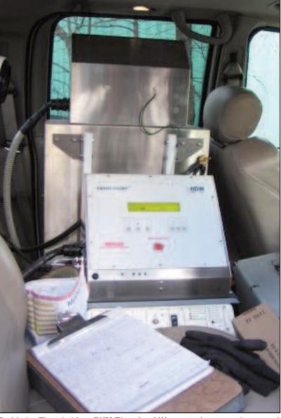
Red Lake Electric hires PKM Electric of Warren to locate underground cable faults. Their truck is equipped with a Smart-Thump thumper and radar unit. Cables from the thumper are hooked to the faulted underground wire and the radar will indicate the approximate footage to where the fault is. The thumper also puts a higher voltage charge onto the wire which will send a shock wave into the ground in the area of the faulted wire.
