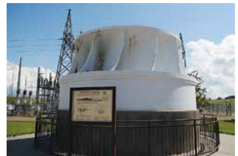
This turbine runner is one of five that were replaced with new stainless steel runners. While in operation, each of the turbine runners power the generators to supply the electrical power needs. The runners were replaced to make the generating unit more dependable and efficient. It is now on display in front of the Garrison Dam power plant.
